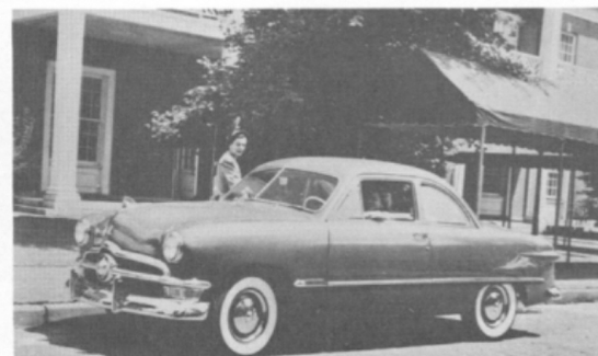
The DeLuxe Business Coupe was a three-passenger car selling for $1,420. Except for wheel and side trim and a non-opening rear quarter window, it was identical to the Custom Club Coupe shown here.
