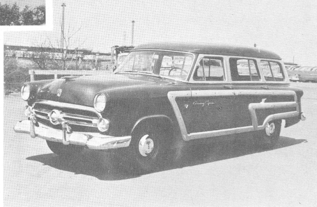
The Country Squire now was an all-steel station wagon with wood veneer trim. Produced as a 4-door model only, it sold for $2,385.
