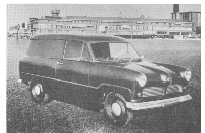
New in Germany was the Taurus 1/2-Ton Van, equipped with a 38 hp, 4-cylinder engine.
